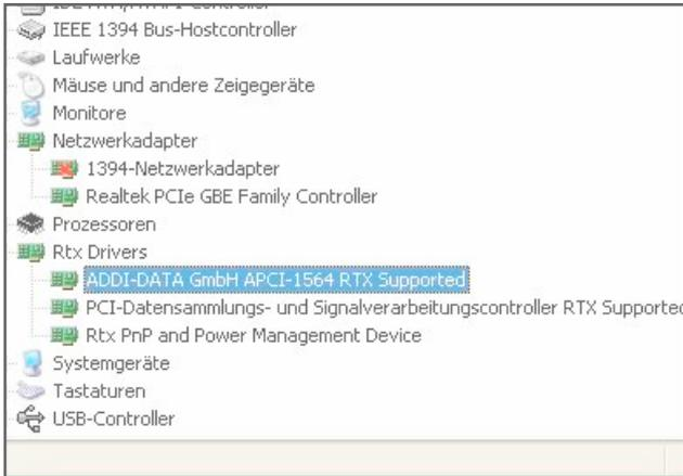
Make sure that the RTX driver of the ADDI-DATA board is installed in the device manager.
