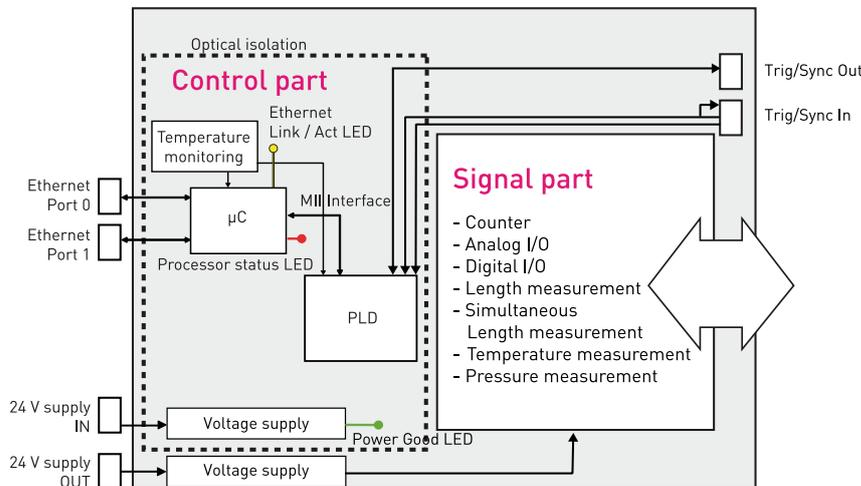
The x-ARTS consist of a signal part and a control part with optical isolation. The real-time connection can be accomplished through EtherCAT, ProfiNet or VARAN. Real-time Ethernet can be used looped-through or as a point-to-point connection.
