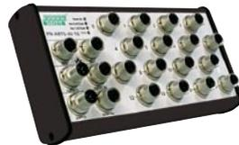
ProfiNet supports both standard Ethernet and real-time connections. It is based on the provider-consumer model, which envisages granting equal rights to the network participants. This model stands in contrast to the standard master-slave process. Not only are process data transferred via ProfiNet, but functions such as web server, e-mail and FTP data transfer are also supported.
