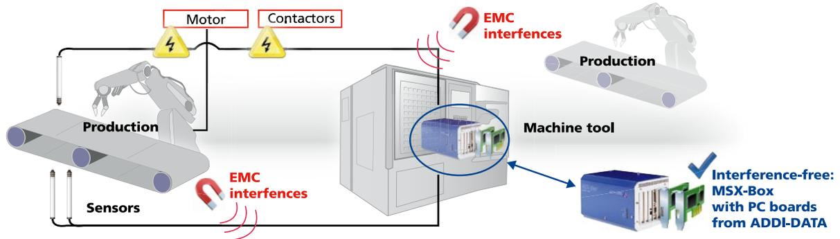
The measurement and control chain is exposed to numerous interfering influences. Measuring errors or even failures may result from the lack of effective protection.
