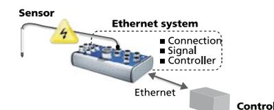
The MSX-Box functions as far as possible without rotating parts, enabling it to be moved closer to the application itself. This distributed use opens up completely new possibilities: The closer the signals measured are to the sensor, the smaller the possible effect of an interference influence on the result. ■
